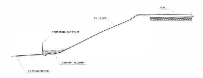
TYPICAL SILT FENCE PLACEMENT
